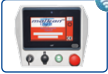
Dokunmatik ekran PLC panel Touch screen PLC
