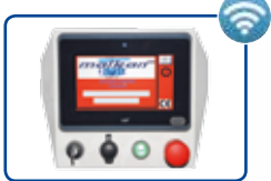
Dokunmatik ekran PLC panel Touch screen PLC
